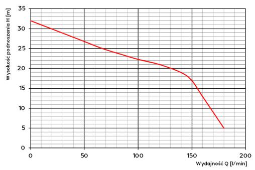
[Rys.: Y: Head max H [m], X: Capacity Q [I/min]]
